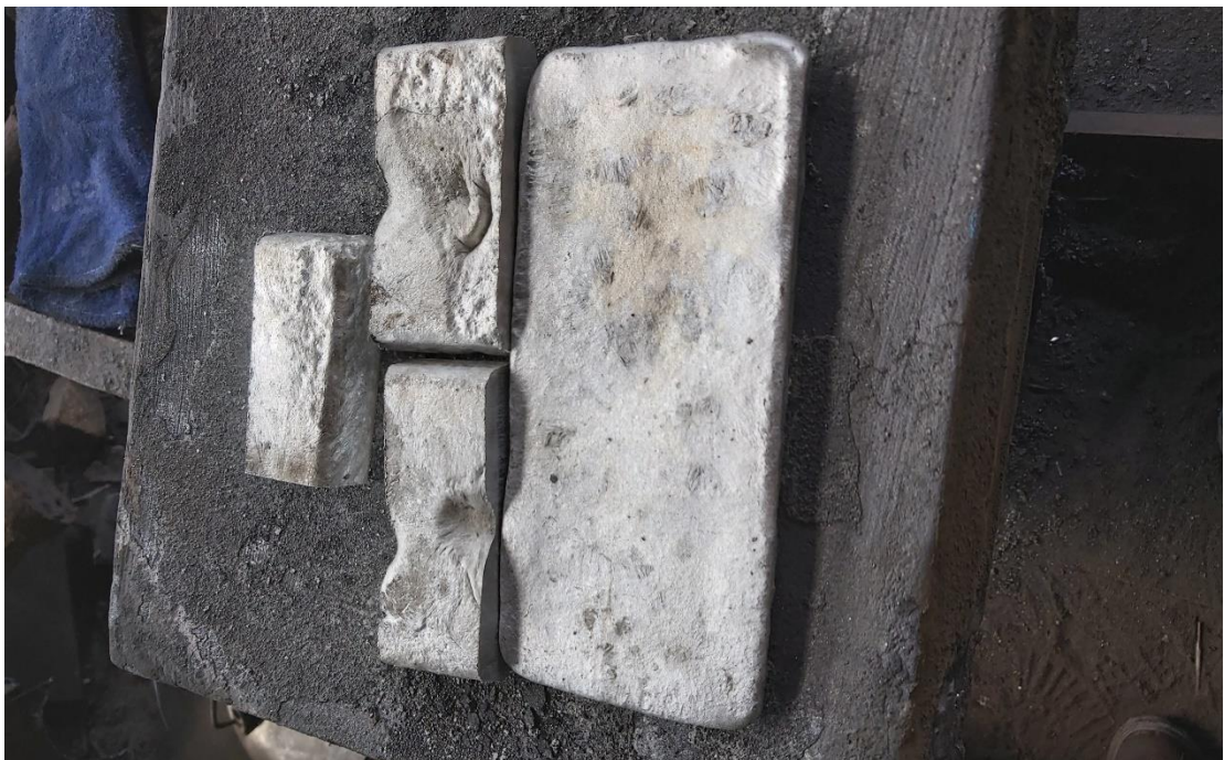
Gambar 52. Aluminium hasil coran
