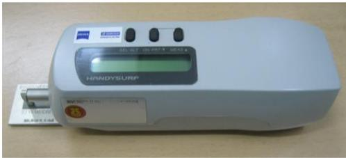
Gambar 4. Handysurf portable surface roughness
