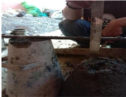
Uji Slump Test
