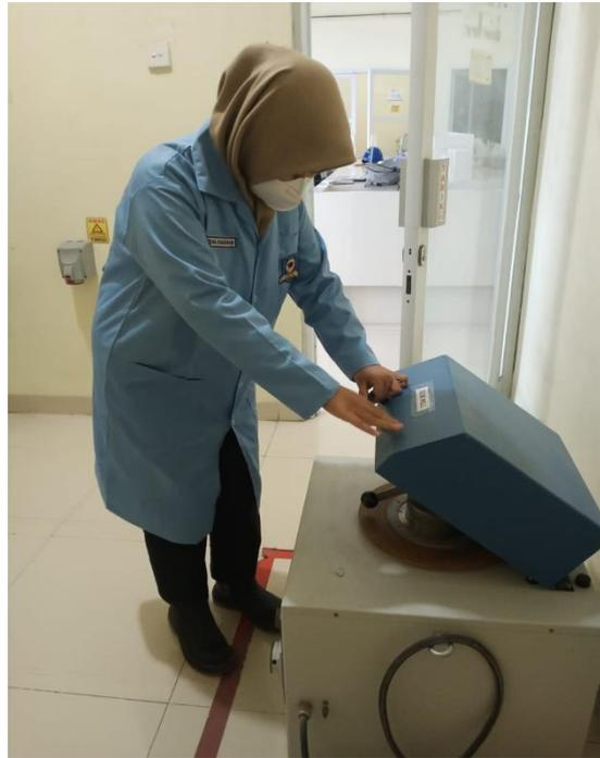
Pembersihan Sampel Dari Grinding Mill
