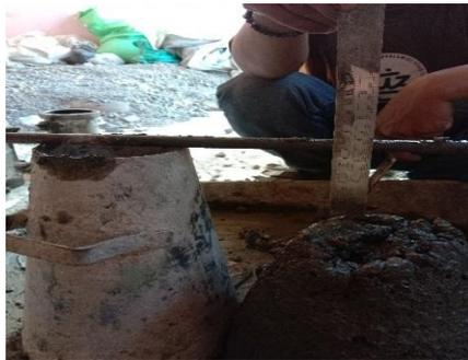
Uji Slump Test
