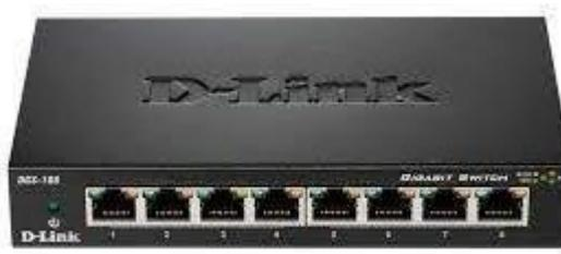
Gambar 2.5 *Switch Unmanageable*
