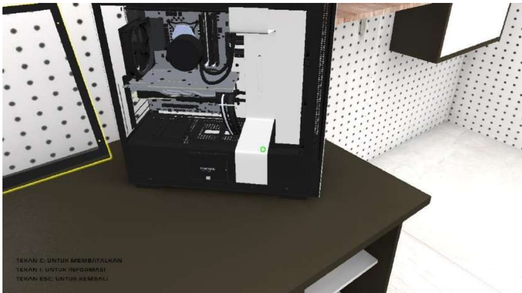
Gambar IV.22 Memasang Power Supply
