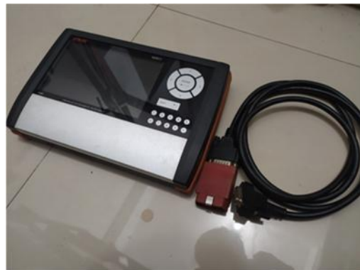
Gambar 3.2. Scanner OBD II
