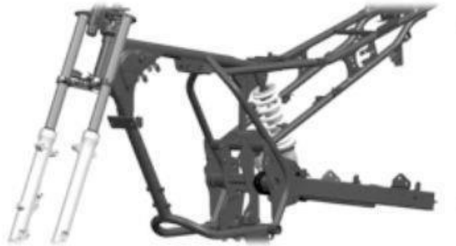
Gambar 2.10 Rangka Half-Duplex cradle (Rangka Bak Semi Model)
