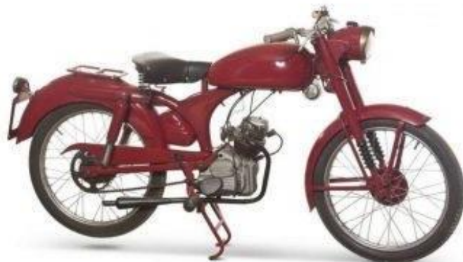
Gambar 2.8 Rangka Pressed (Rangka Press)
