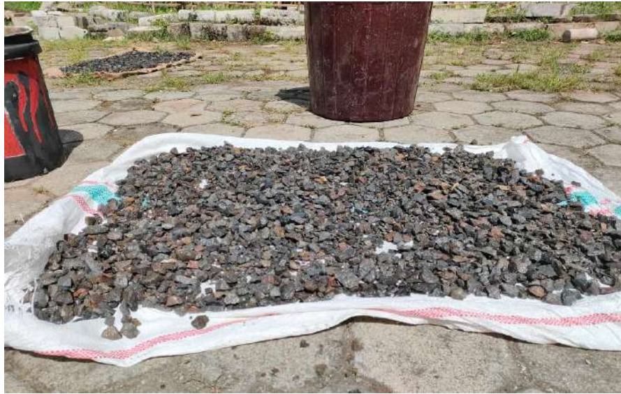
Penjemuran agregat kasar (chipping)
