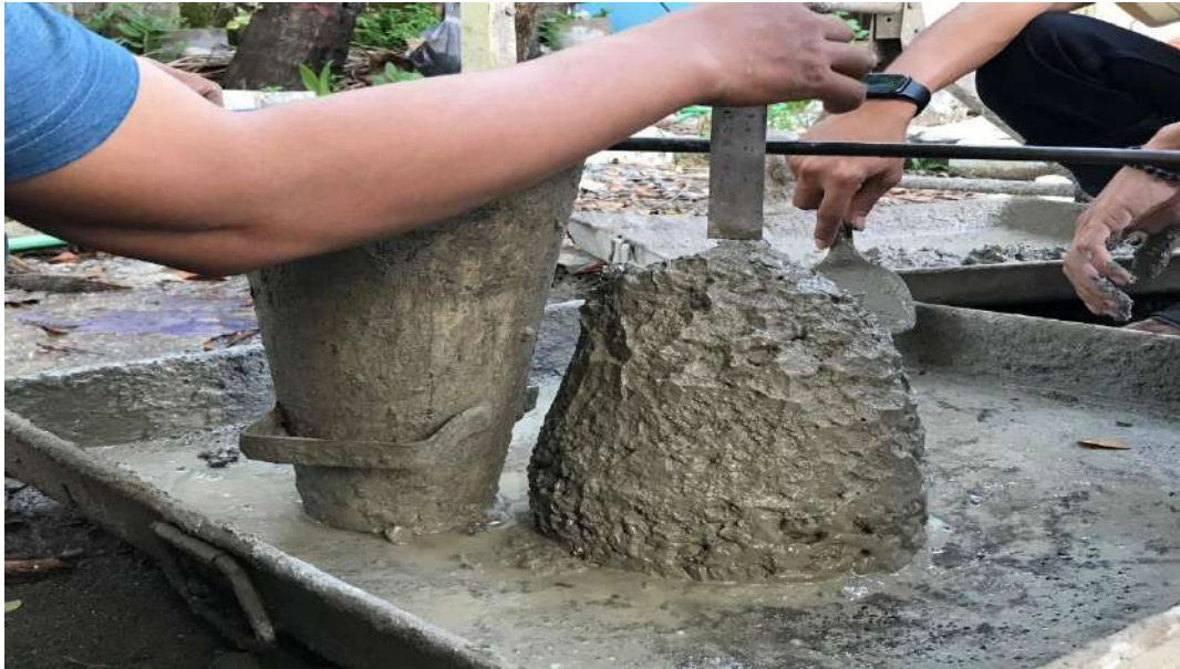
Proses Slump Test Beton
