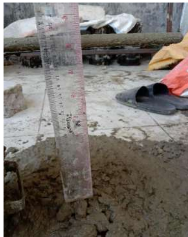
Gambar IV.6 Pengujian Slump Variasi Fly Ash 15%
