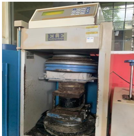
Gambar III. 1 Pengujian Kuat Tekan Paving Block
