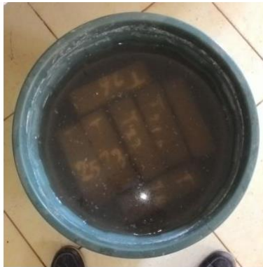
Gambar III. 2 Perendaman Sampel Paving Block.
