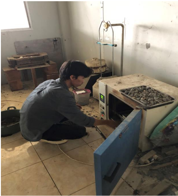
PROSES OVEN BENDA UJI
