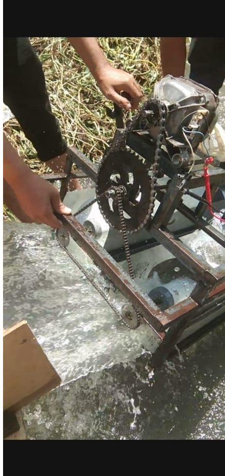
Gambar IV.1 Prototype Turbin Air Dual Screw Kapasitas 100 Watt
