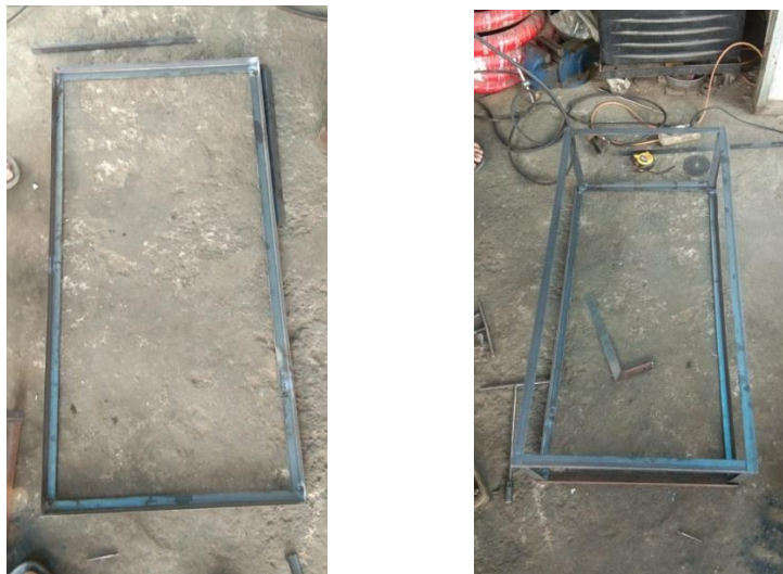
Gambar IV.3 Rangka Prototype Turbin Air Dual Screw
