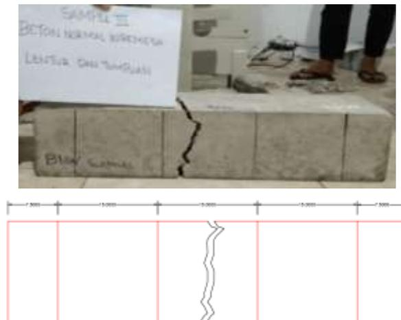
Gambar IV. 10 Pola Retak Beton Wiremesh (BNW<sub>3</sub>)
