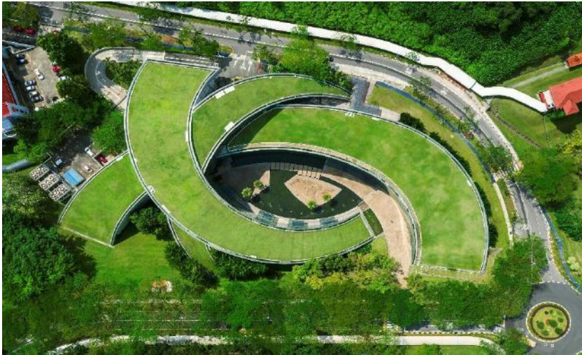
Gambar 9.1. Aplikasi Green Roof pada Kampus NTU School of Art, Design and Media (Nur'aini, 2017)
