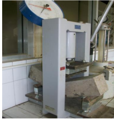
Figure 4. Flexural Strength Test
