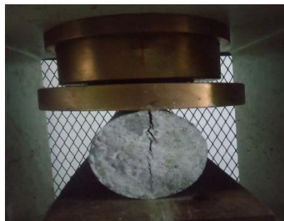
Figure 3. Split Tensile Strength Test
