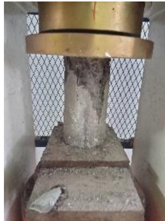
Figure 2. Compressive Strength Test
