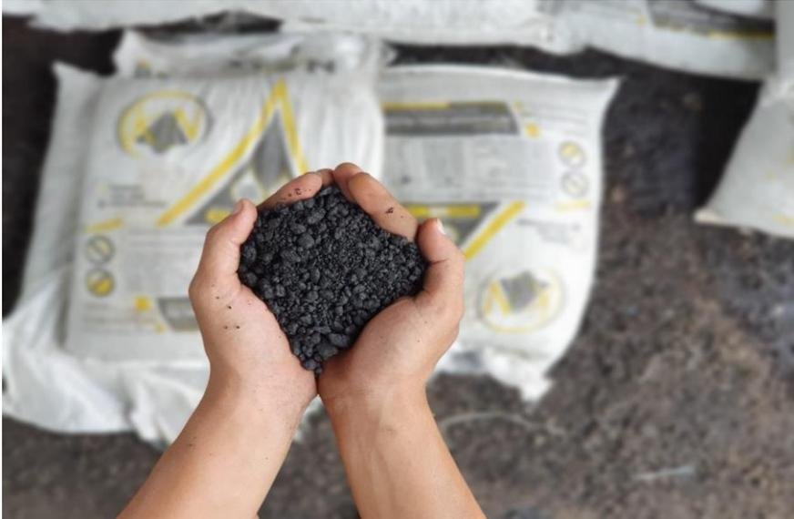
**Gambar 7.1** Visual Perkerasan CPHMA
