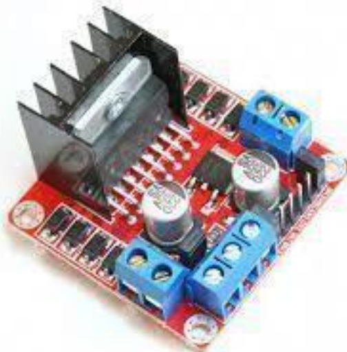
Gambar II.3 Motor Driver (Sumber : Mutaqqin, 2021)
