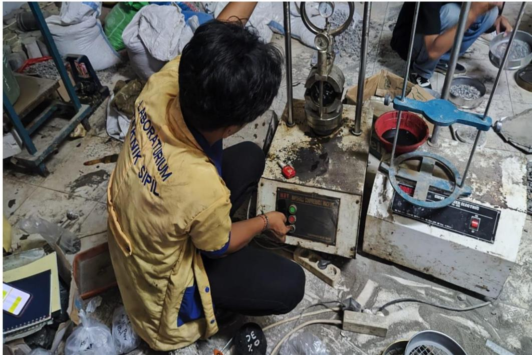
Pengujian Marshall (Marshall Compression)
