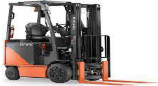
Gambar 2.7 Forklift energi listrik Sumber (Suganda, 2019)
