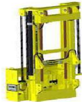
Gambar 2.10 Mast Forklift (Suganda, 2019)
