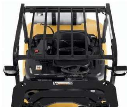
Gambar 2.11 Overhead Guard Forklift (Suganda,2019)
