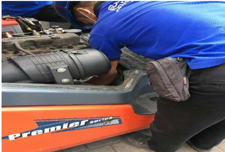
Gambar 14. Proses Pengantian Dinamo Stater Forklift 3 Ton
