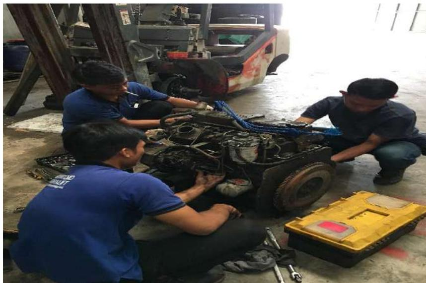
Gambar 20. Proses Overhaul Pada Mesin Forklift 3 Ton
