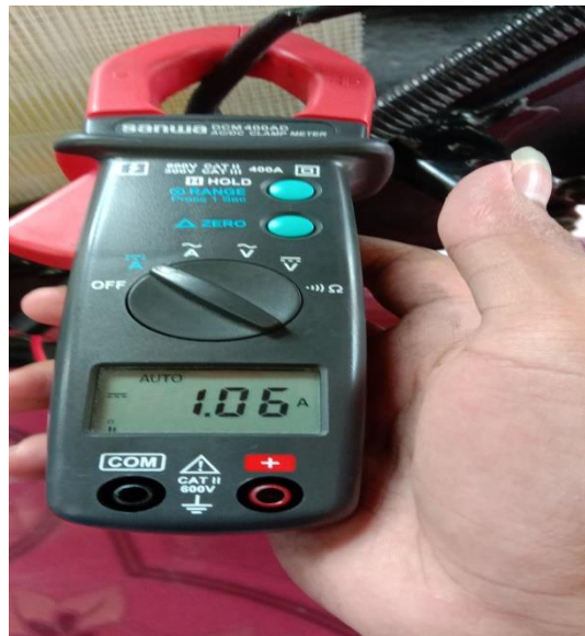
Gambar III.4. Clamp meter/ tang meter
