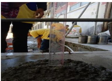
Gambar IV. 4 Pengujian Slump Variasi Fly Ash 0%
