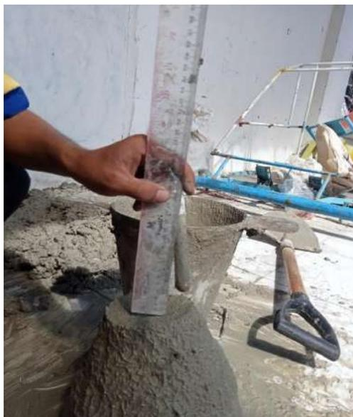
**Gambar IV.1 Slumpt Test**
