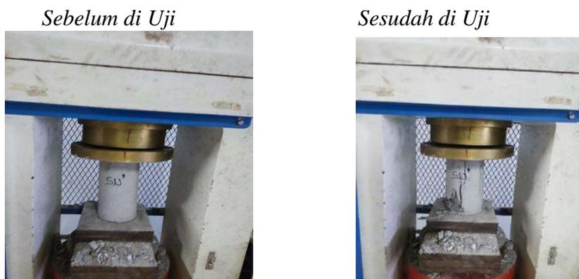
Gambar IV 1 Pengujian Kuat Tekan Beton Silinder Normal (SN)
