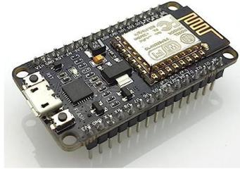
**Gambar 2.3 NODEMCU Esp2866**
