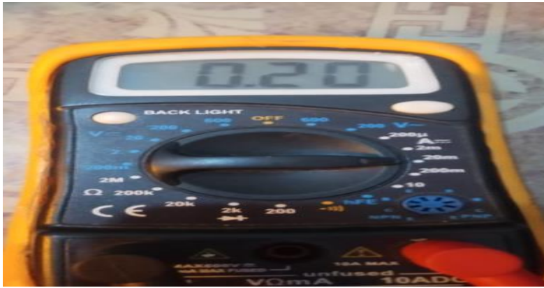
6. Tegangan output led 2,4 watt
