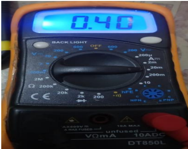
4. Tegangan output led 3 watt
