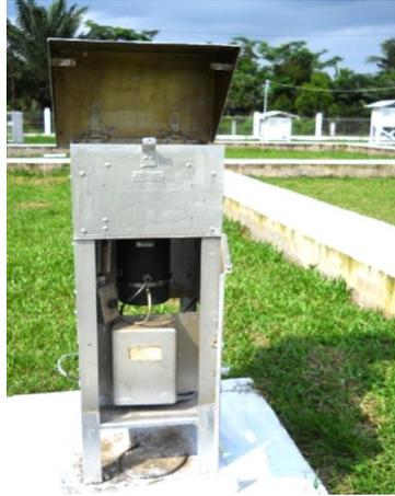
**Gambar 5.7** High Volume Air Sampler (BMKG, 2022)
